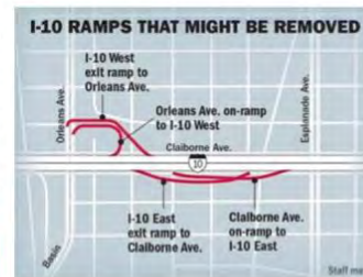
LADOT Concept Removing Four Ramps
