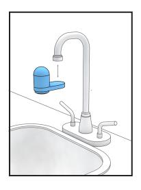
The filter connects to the faucet using an adapter.
